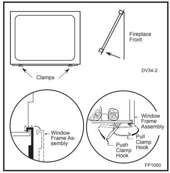
Fig. 13 Window Frame installation and removal.
